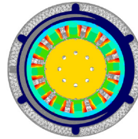
Electric motor thermal simulation
