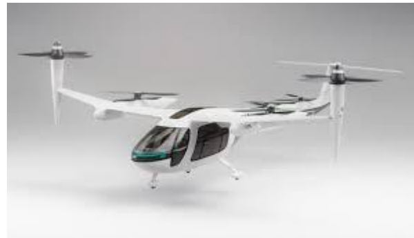
Fig. 2: Uber Elevate eCRM001 eVTOL Configuration
